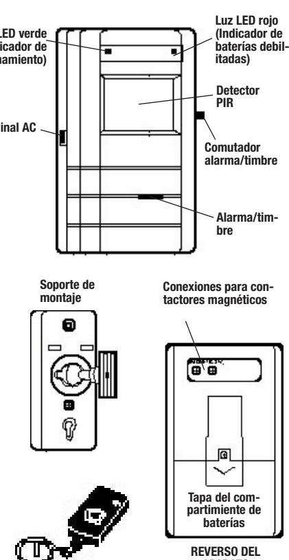
equipped with terminales for use with magnetic contacts. Magnetic contacts can be purchased separately.
